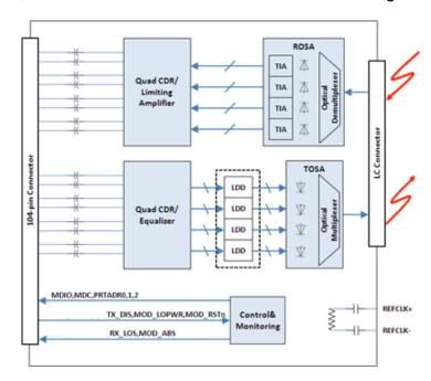
Figure 1. CFP4 LR4 Optical Transceiver functional block diagram
